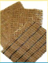
such as coir (coconut) and straw, which are supported and interwoven with either jute or polypropylene netting. These products help to successfully establish vegetative growth on slopes and embankments before naturally breaking down and becoming part of the established vegetation.
